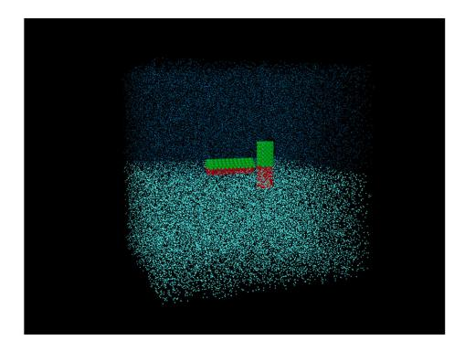
Janus rods with the same surface characteristics except for the geometry of the coating are depicted. The particles assume completely different orientations, implying they also assume different mechanical properties for the overall interface. Credit: Giovanniantonio Natale
