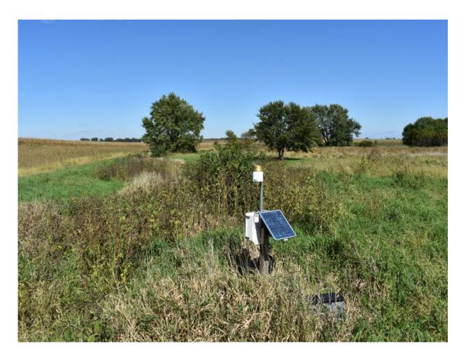
A solar-powered data logger measures water levels at an experimental saturated riparian buffer. It was installed by a team from Iowa State, whose research determined criteria that show more farmland qualifies to safely install riparian buffer strips. Credit: Loulou Dickey
