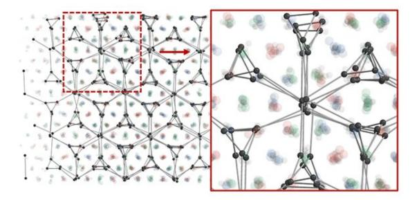
This triple-double gyroid is a new colloidal crystal structure that has never been found in nature or synthesized before. The translucent red/green/blue balls show the positions of programmable atom equivalents (PAEs), while the dark grey balls and sticks show locations of electron equivalents (EEs). Credit: Sangmin Lee
