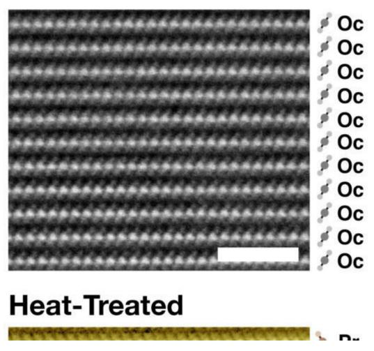
This electron microscopy image shows the atoms within individual twodimensional layers of tantalum sulfide before and after the heat treating process. Before heat-treating, all layers are bonded with octahedral geometry. After heat-
