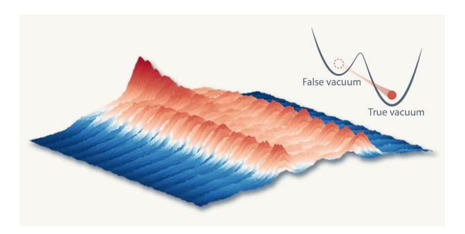
Measured momentum distribution of the shaken quantum gas during the phase transition. The central peak on the left corresponds to the initial Mott insulator while the two peaks on the right indicate the appearance of the distinct staggered order. Credit: Bo Cheng
