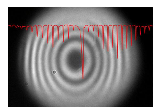
The invisible made visible: Using entangled photons and interference effects, infrared spectra of molecules (here: methane) can be recorded by cameras that can only detect visible light. Credit: Fraunhofer IPM
