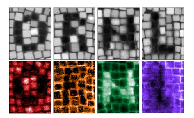
ORNL scientists used an electron beam for precision machining of nanoscale materials. Cubes were milled to change their shape and could also be removed from an array. Credit: Kevin Roccapriore/ORNL, U.S. Dept. of Energy
