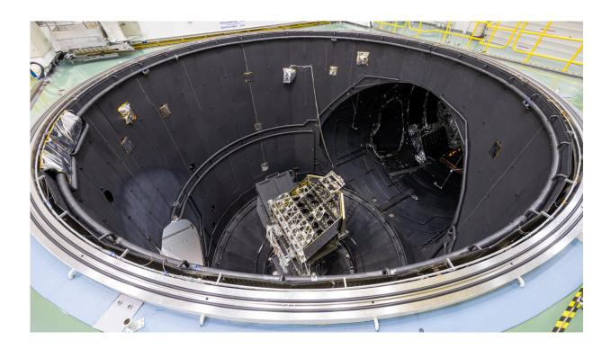
Plato optical bench entering the Large Space Simulator (ESTEC) for the thermoselastic deformation test (TED) in September 2021. Credit: European Space Agency
