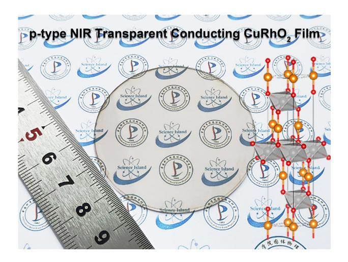
Fig. 1. Photo of p-type NIR TCCuRhO2 thin film with 2 inches size. Credit: Wei Renhuai
