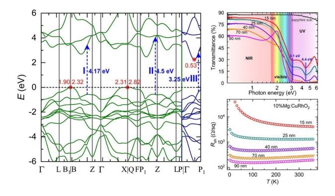
Fig. 2. Calculated electronic band structure for the  $CuRhO_2$  (left).Optical transmittance and room-temperature sheet resistance for 10% Mg-doped  $CuRhO_2$  thin films (right). Credit: Wei Renhuai
