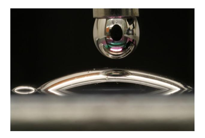
Researchers can now treat a surface so that a droplet of mercury spreads out on it, instead of beading up. Credit: Massachusetts Institute of Technology
