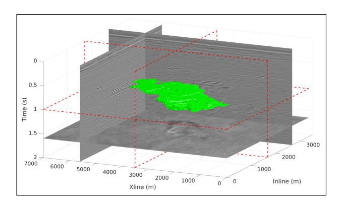
In this 3D seismic observation, the carbon dioxide (CO2) reservoir has been labeled in green by a human evaluator, but according to a new study, machine learning algorithms may soon replace people for this task. Credit: DOI: 10.1029/2021JB022524
