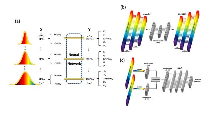
Fig.2. (a) Mapping between spectrum and laser parameters used for neural network training, (b) (c) the structures of the neural network. Credit: Institute of Physics
