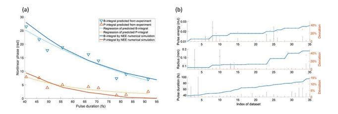
Fig. 3. Comparison of the prediction of B, P integrals and the initial pulse parameters based on neural network with experimental results. Credit: Institute of Physics
