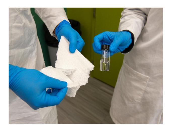
A multi-institute research team used hairy cellulose nanocrystals, developed from the main component of plant cell walls and used in a variety of materials, including paper, to capture off-target chemotherapy drugs to prevent tissue damage. Credit: Kate Myers/Penn State
