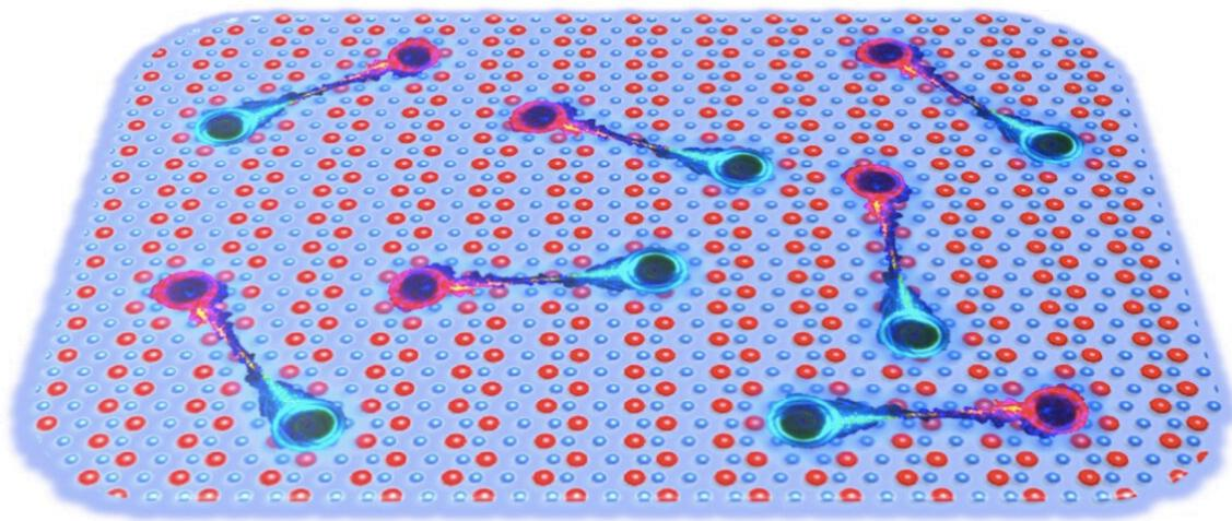
Cartoon illustration of the excitonic insulator formed in the single atomic layer of tungsten ditelluride. The excitons are charge neutral composite particles like the hydrogen atoms, hidden in the two-dimensional electrical insulator. Credit: Wu Lab, Princeton University.
