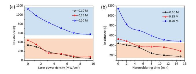
Fig. 2. (a) Measured resistance of the Ag NWs electrodes as a function of the laser nanosoldering power density with the laser nanosoldering time of 11 min. (b) Measured resistance of the Ag NWs electrodes as a function of the laser nanosoldering time with laser nanosoldering power density of 7.01 MW/cm<sup>2</sup>. Credit: Compuscript Ltd
