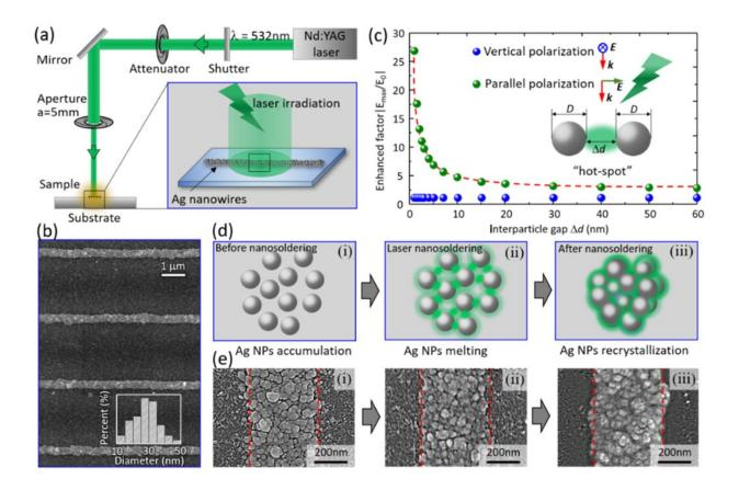
Fig. 1. (a) Schematic of experimental system for PLNS. (b) Scanning electron microscope (SEM) image of Ag NWs with inset showing the size distribution of Ag NPs in Ag NWs. (c) Plasmon-enhanced electric field as a function of interparticle gap for light polarization direction parallel and vertical to the interparticle axis. (d) Schematic illustration of PLNS with increasing laser irradiation time. (e) SEM images of the morphological changes of Ag NWs in
