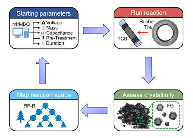
Machine learning is fine-tuning Rice University's flash Joule heating method for making graphene from a variety of carbon sources, including waste materials. Credit: Jacob Beckham
