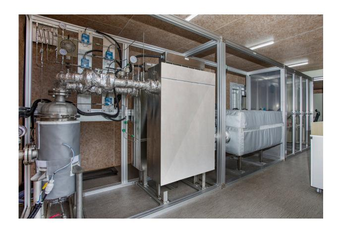
SCR pilot DeNOx reactor through on-site exhaust gas injection. Credit: Korea Institute of Science and Technology(KIST)
