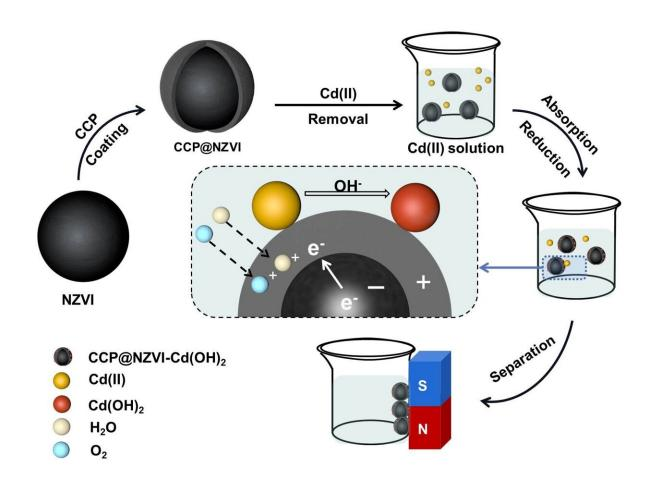
Schematic illustration of removal mechanism. Credit: Guo Xinyue
