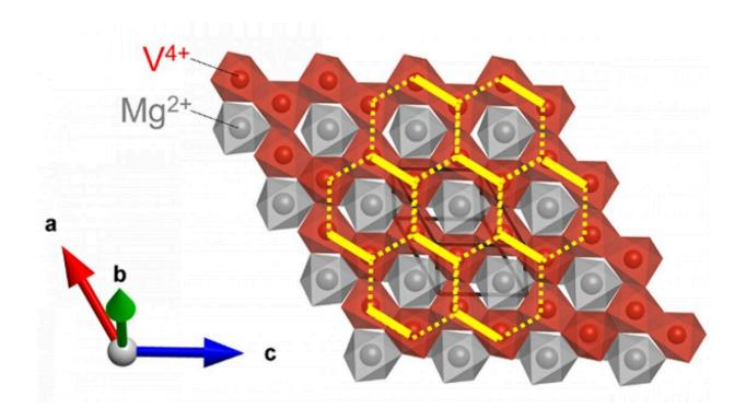
The crystal structure of ilmenite-type magnesium vanadate (MgVO3). The yellow line shows the honeycomb lattice. The thick lines indicate the location of V-V dimers. The crystal structure was drawn using VESTA-3 software. Credit: Hajime Yamamoto
