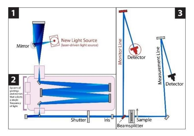
The transmittance calibration set-up has three parts: (1) the source (upper left corner), which in this case is a laser-driven light source that produces UV light; (2) the monochromator, which uses gratings and mirrors to let researchers select a particular wavelength; and (3) the detectors that allow researchers to determine how much light transmits through the sample. Credit: National Institute of Standards and Technology
