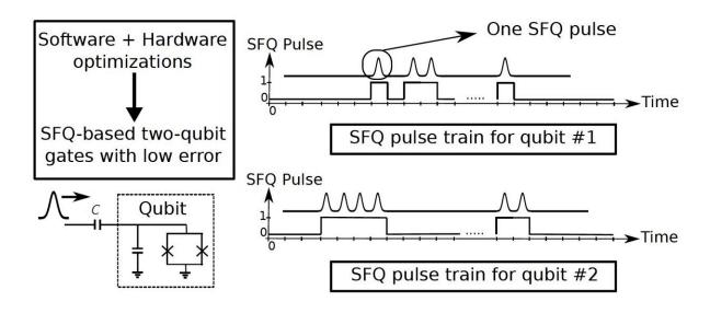
A new hardware/software strategy for realizing low-leakage SFQ-based twoqubit gates could help overcome a major scalability obstacle for today's quantum computers. Credit: University of Chicago/EPiQC
