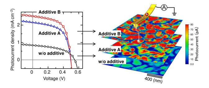
Improvements in the device performance by addition of a solvent additive A and B (left). Photocurrent flowing in the polymer solar cells, which is visualized at nanometer scale by PC-AFM (right). Credit: Nara Institute of Science and Technology
