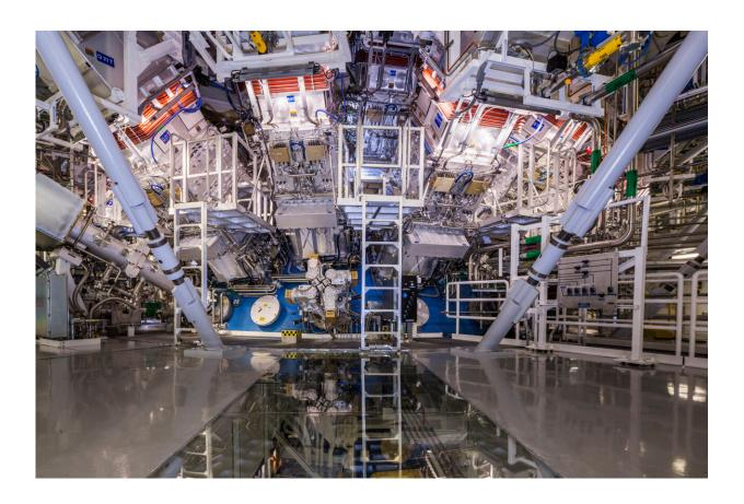
This image provided by the National Ignition Facility at the Lawrence Livermore National Laboratory shows the NIF Target Bay in Livermore, Calif. The system uses 192 laser beams converging at the center of this giant sphere to make a tiny
