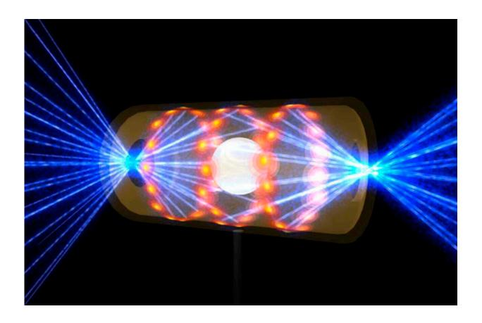
This illustration provided by the National Ignition Facility at the Lawrence Livermore National Laboratory depicts a target pellet inside a hohlraum capsule with laser beams entering through openings on either end. The beams compress and heat the target to the necessary conditions for nuclear fusion to occur. Credit: Lawrence Livermore National Laboratory via AP
