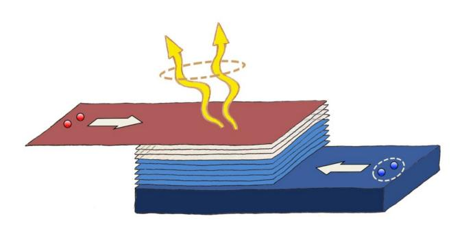
Schematic view of the entangled photon generator. The dark blue bottom layer is a superconductor from which the paired, entangled electrons tunnel through the light blue layered structure to the upper layers. The entangled photon pair is created, when the tunneled electrons make a transition to empty lower energy levels simultaneously. Credit: Ethan D. Minot
