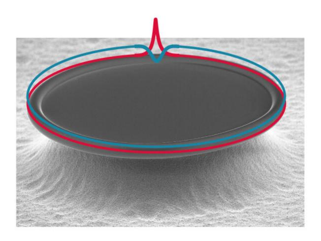
Visualisation of coupled dark and bright light pulses (blue and red respectively) in a microresonator, which has a diameter of 235 micrometer. Credit: Max-Planck-Institute for the Science of Light
