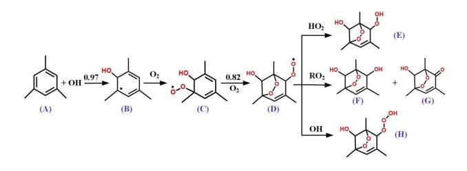
Fig. 1 The major reaction routes of the OH initiated photo-oxidation of 1,3,5-TMB under NOx free conditions. Credit: Lin Xiaoxiao
