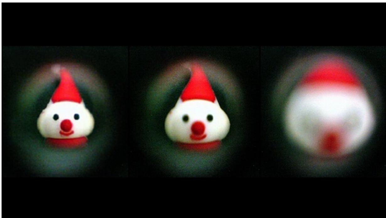
Researchers developed an adaptive liquid lens based on a new electrically responsive fluid called dibutyl adipate (DBA). The new lens changes shape, and thus focal length, when a voltage is applied. Credit: Miao Xu, Hefei University of Technology
