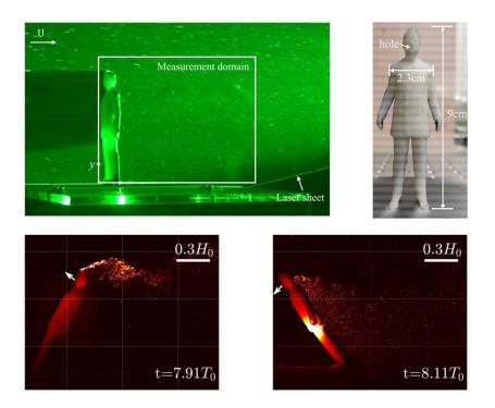
Experimental fluid mechanics show the different patterns of droplets dispersion from a person going up or downstairs corresponding to the wake flow. Credit: Hongping Wang
