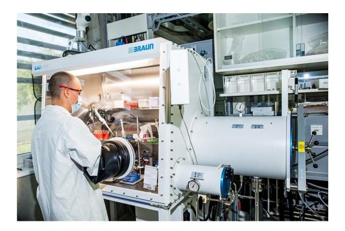
In the "glovebox", the functionality of the enzymes is monitored electrochemically in the absence of air. Credit: Fraunhofer Institute for Interfacial Engineering and Biotechnology IGB
