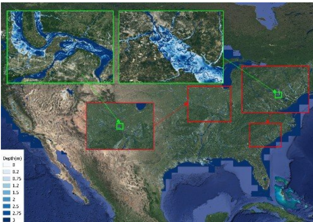
The nationwide simulation of the 100-year design flood from fluvial, pluvial, and coastal sources. Credit: Fathom (fathom.global)
