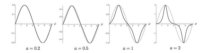
Fig. 1: Sine wave curvatures and capillary non-linearity. Comparison of dimensionless in-plane curvatures [solid curves from Eq. (2)] shown with their profiles (broken curves). Profiles are plotted non-isometrically. Note the scale change on the ordinates with increasing amplitude, a Higher harmonic content of the curvature distribution is nearly absent at low wave amplitudes, a 0.5. Credit: DOI: 10.1038/s41526-021-00168-2
