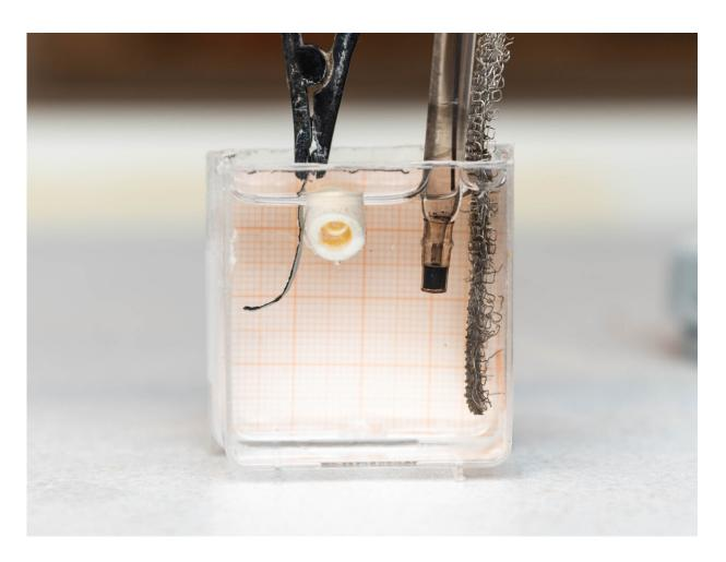
When voltage is applied, the material (left) will slowly bend towards the chicken bone (white). If the liquid contains the minerals needed for bone development, the material will, in the space of a few days, begin to build artificial bone that attaches itself to the chicken bone. Credit: Olov Planthaber/LiU
