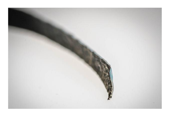
The black material is an electroactive polymer, the volume of which changes when the researchers apply a low voltage, which makes this simple "microrobot" bend. On the other side of the material, you can see the gel to which the researchers have attached biomolecules that allow the soft gel material to harden like a bone. Credit: Olov Planthaber/LiU
