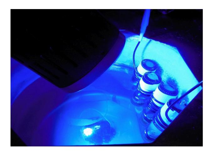
Reaction vials being exposed to blue light from an LED. Credit: Yusuke Masuda
