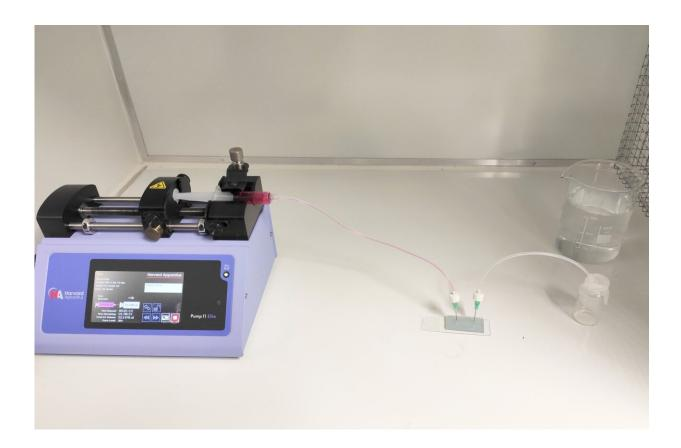
The biochip enables in vitro skin culture to be grown inside the biochip. The flows are controlled by highly accurate syringe pumps. Credit: UC3M
