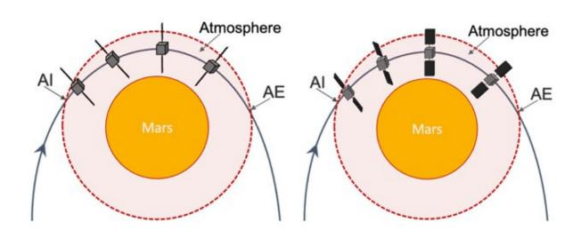
Representation of (a) current aerobraking with static, perpendicular solar panels, and (b) the proposed concept using rotating solar panels to actively control the trajectory. Credit: University of Illinois Dept. of Aerospace Engineering
