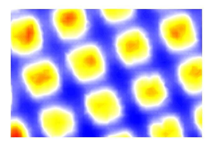
The image of the graphene layers on the photocathode shows areas of low quantum efficiency (in blue) where no electron transmission occurs. The red and yellow areas show increasingly high quantum efficiency. Photoelectrons are emitted and transmitted through the graphene in those areas while overall the material is protected from corrosive gases produced. Credit: Los Alamos National Laboratory
