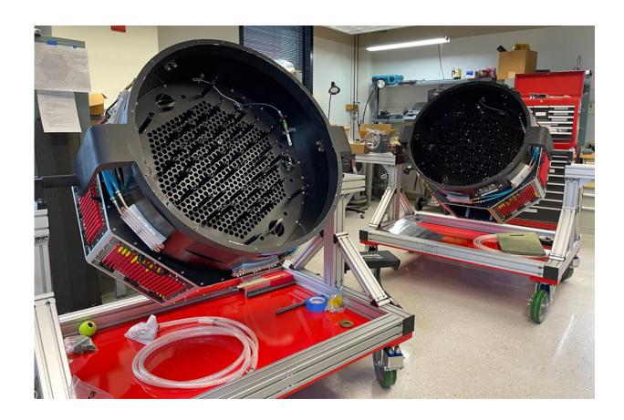
The Focal Plane System replaces a time-consuming, hands-on approach to making simultaneous observations of hundreds of stars. Credit: SDSS-V
