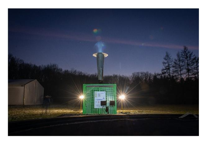
The experimental sound "cannon", which Polish researchers say can blast toxic particles hundreds of metres into the sky.
