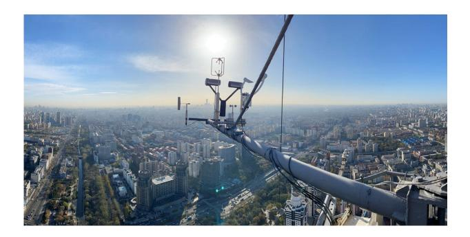
A photo of haze over Beijing. Also shown are the instruments of four-cup anemometers, meteoprobe, ultrasonic anemometer and visibility meter installed on the Beijing 325 m meteorological tower. Credit: Li Hao
