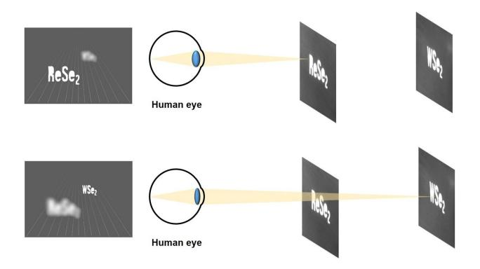
Hologram implemented with two-dimensional semiconductor WSe2/ReSe2, which is a polarization-sensing photodiode, ReSe2 on the front and WSe2 on the back are imaged in three-dimensional space. Credit: Korea Institute of Science and Technology (KIST)
