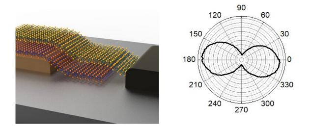
3D device schematic of a 2D WSe2/ReSe2 pn heterojunction photodiode (left) and photocurrent modulation as a function of linear polarization angle of incident light (right). Credit: Korea Institute of Science and Technology (KIST)
