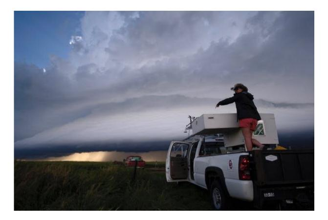
A researcher with NOAA and the Oklahoma Cooperative Institute prepares a light detection and ranging system to collect data at the edge of a storm. Credit: Mike Coniglio/NOAA NSSL
