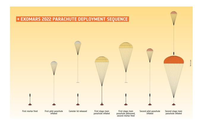
The ExoMars parachute deployment sequence that will deliver a surface platform and rover to the surface of Mars in 2023 (following launch in 2022). The graphic is not to scale, and the colours of the parachutes are for illustrative purposes only. Credit: European Space Agency
