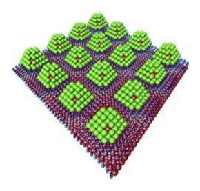
The palladium nanoparticles (green) are stabilized by a core of iridium (red). Hydrogen can accumulate on their surface like a kind of chocolate glaze—and can be released again by heating. Credit: DESY, Andreas Stierle
