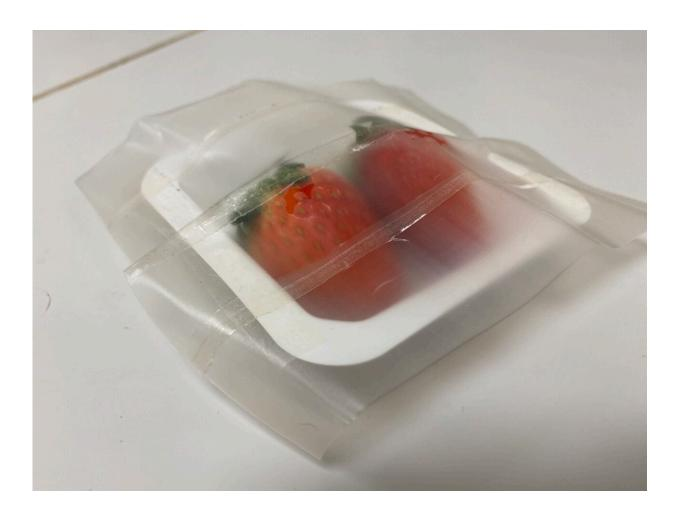
In an experiment, strawberries that were wrapped in the NTU-Harvard University-developed packaging stayed fresh for seven days before developing mould, compared to counterparts that were kept in mainstream fruit plastic boxes, which stayed fresh for four days. Credit: Nanyang Technological University
