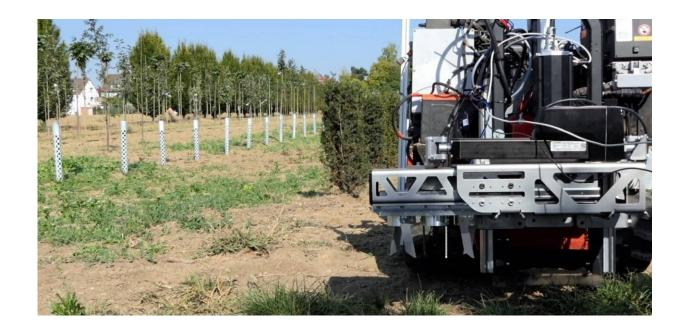
The manipulator also moves in the gaps between the crop rows and removes any weeds here using the rotary harrows. Credit: Federal Office of Agriculture and Food/Fraunhofer
