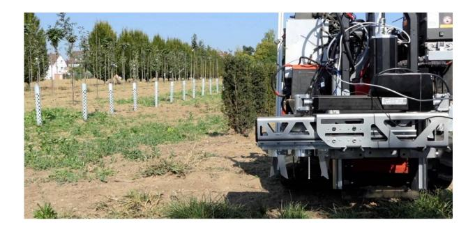
The manipulator also moves in the gaps between the crop rows and removes any weeds here using the rotary harrows. Credit: Federal Office of Agriculture and Food/Fraunhofer
