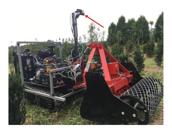
The LiDAR scanner (red arrow) installed in AMU-Bot continuously emits laser pulses as the vehicle moves, which the system uses to determine the position of the crop rows. Credit: Federal Office of Agriculture and Food/Fraunhofer
