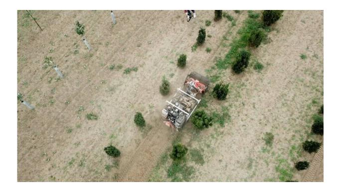
The autonomous caterpillar vehicle, AMU-Bot, drives between the rows in the tree nursery and removes any weeds. Credit: Federal Office of Agriculture and Food/Fraunhofer
