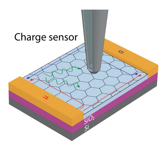
A charge sensor measuring the cost of electrons surfing on the spin wave (green
