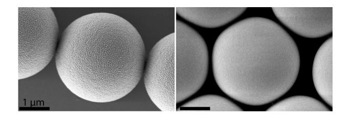
Electron micrographs of polystyrene particles of the same name from two different manufacturers. They show different surface morphologies that can lead to different cell interactions. Credit: Julia Jasinski
