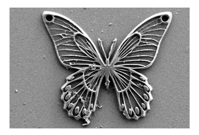
A micro-butterfly, printed by Del Pozo. The width is around 70 micrometers. Credit: Eindhoven University of Technology
