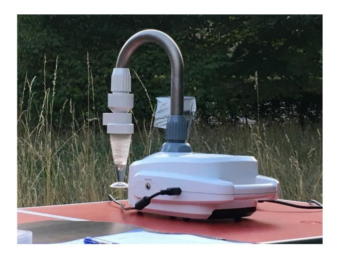
Coriolis  $\mu$ . The air sampler used to obtain eDNA from insects in the field. It works by sucking in air and swirling it through water, where the particles contained in the air get captured. Credit: Fabian Roger
