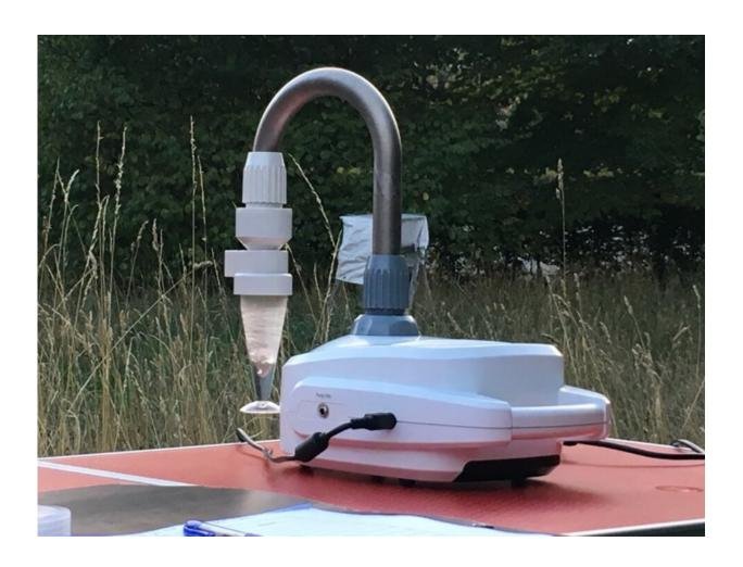
Coriolis  $\mu$ . The air sampler used to obtain eDNA from insects in the field. It works by sucking in air and swirling it through water, where the particles contained in the air get captured. Credit: Fabian Roger
