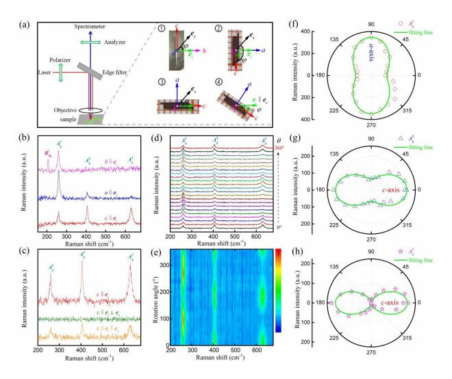
Fig. 2. 3D anisotropic phonon vibration of MoAlB single crystal. Credit: Huang Yanan
